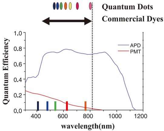
Quantum Efficiency for the R3896 PMT and the RMD avalanche photodiode (APD) as a function of wavelength.
