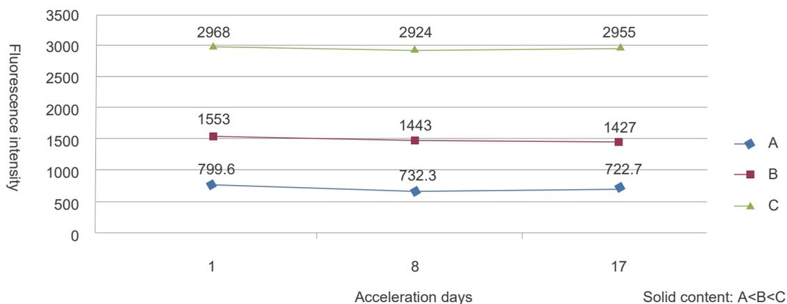
▲ After accelerating at 37°C for 17 days, there was no significant change in the fluorescence intensity of the time-resolved fluorescent microspheres solutions with different solid contents, and the microspheres shows high stability.
