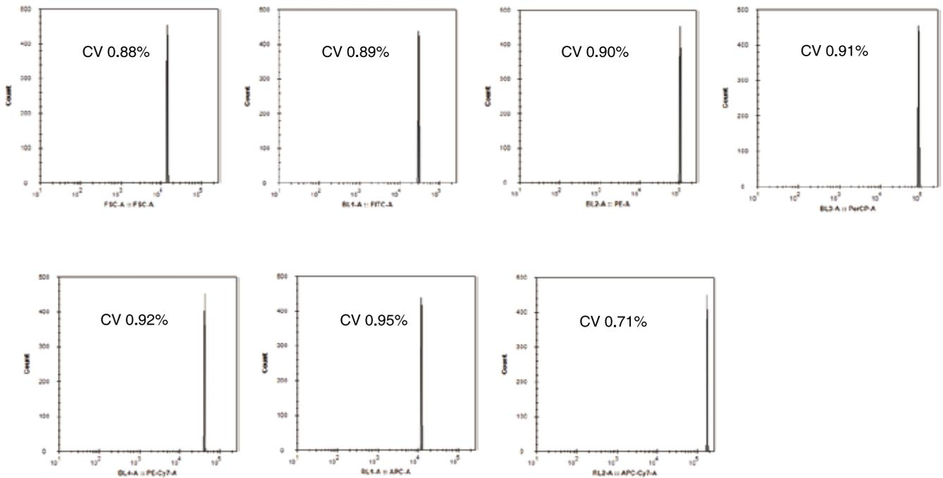
Based on the resolution detection of Spherotech UFRP302 Rainbow Single Peak microsphere, CVs of all channels are less than 2%
