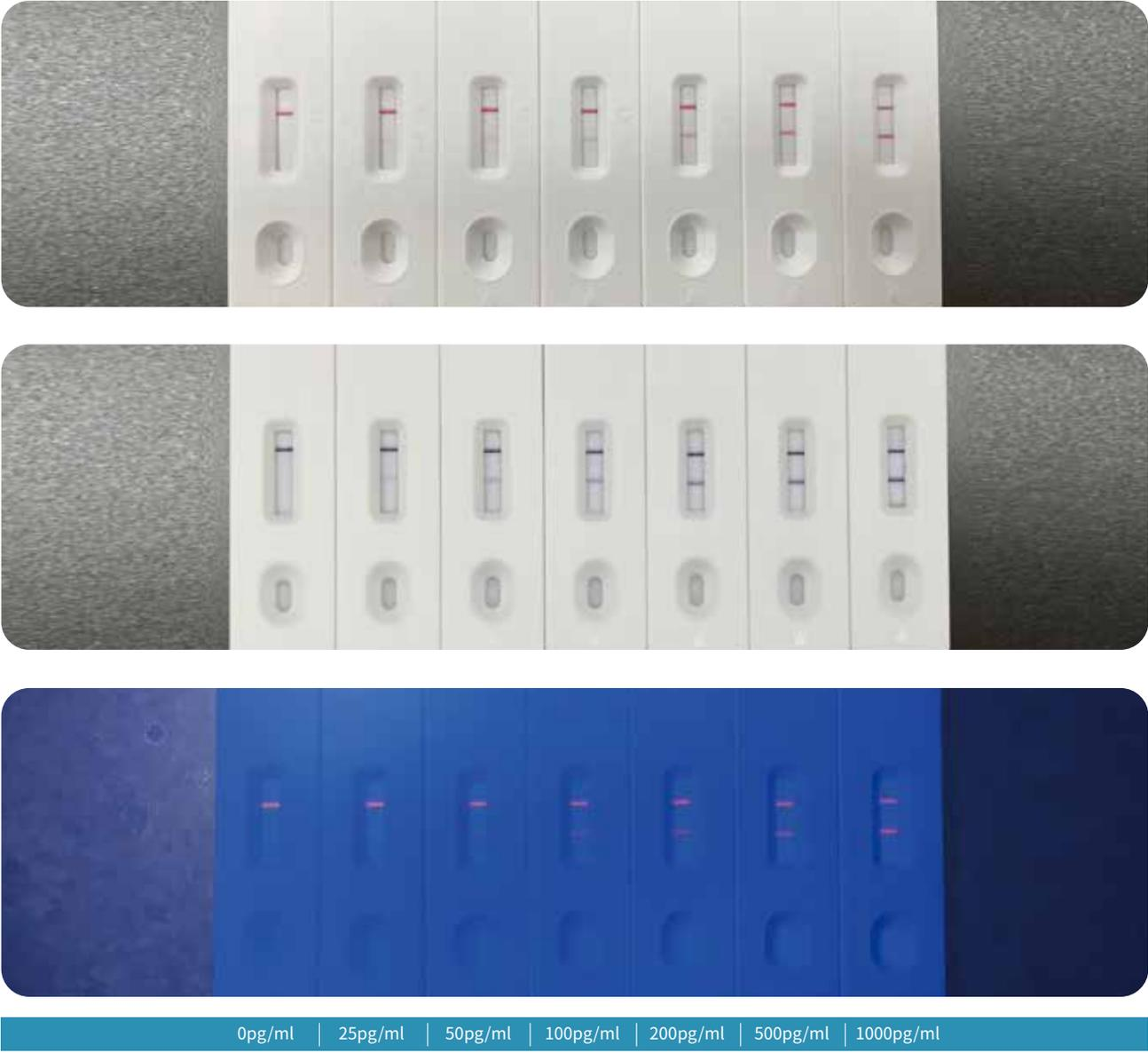
▲ SARS-CoV-2 N protein was detected by VDO Biotech's color-dyed microspheres and fluorescent microspheres respectively, and the protein can still be detected when the concentration is as low as 25pg/ml.
