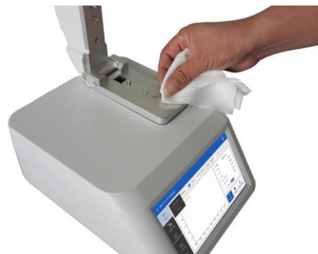
Fig 3.4 Clean upper and lower pedestal
